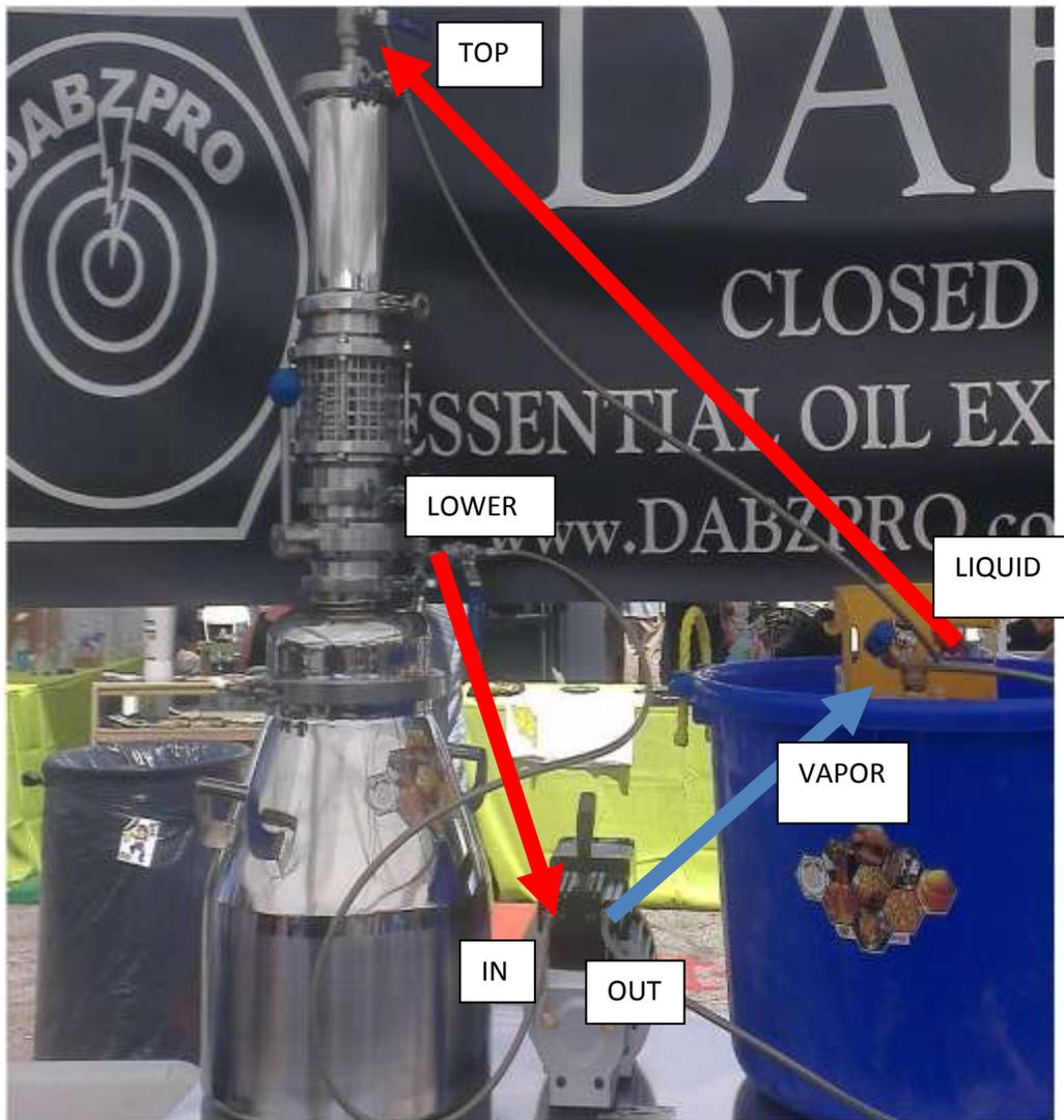
1. First the 6cfm **purge** pump is applied to get the collection tank of the extractor down to -30hg the max allowed in space.
