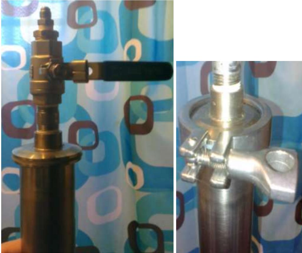
Place the top and attach with a clamp. The Extractor is ready to be hooked up to the Re-Claim System.
