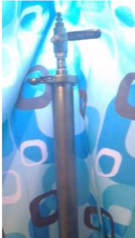
7. Open the **Vapor** handle on the LP5 Butane Tank this is where the butane gas gets collected back into.
